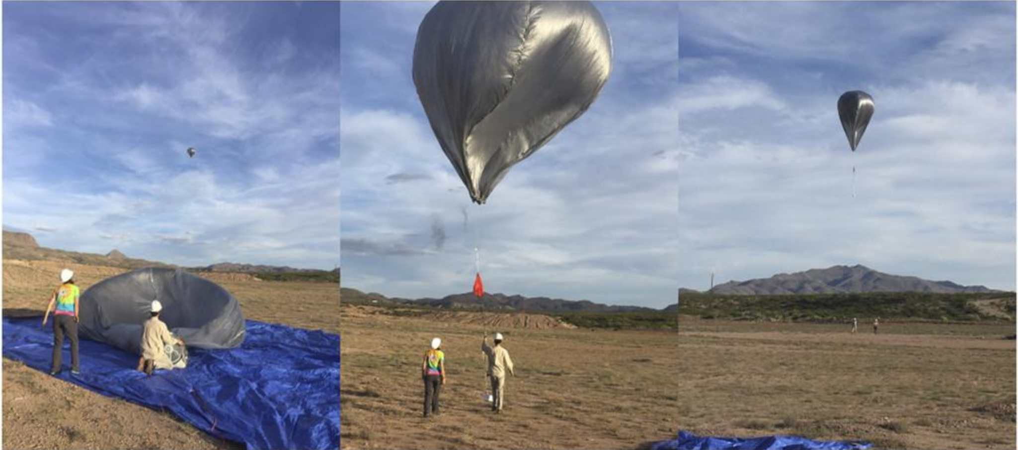
Figures: (left) Inflating a 6 m heliotrope with a box fan, (center) walking the inflated envelope across an open area until it gains sufficient lift to pick up the payload, and (right) a successful launch. ( Bowman, 2020 )
